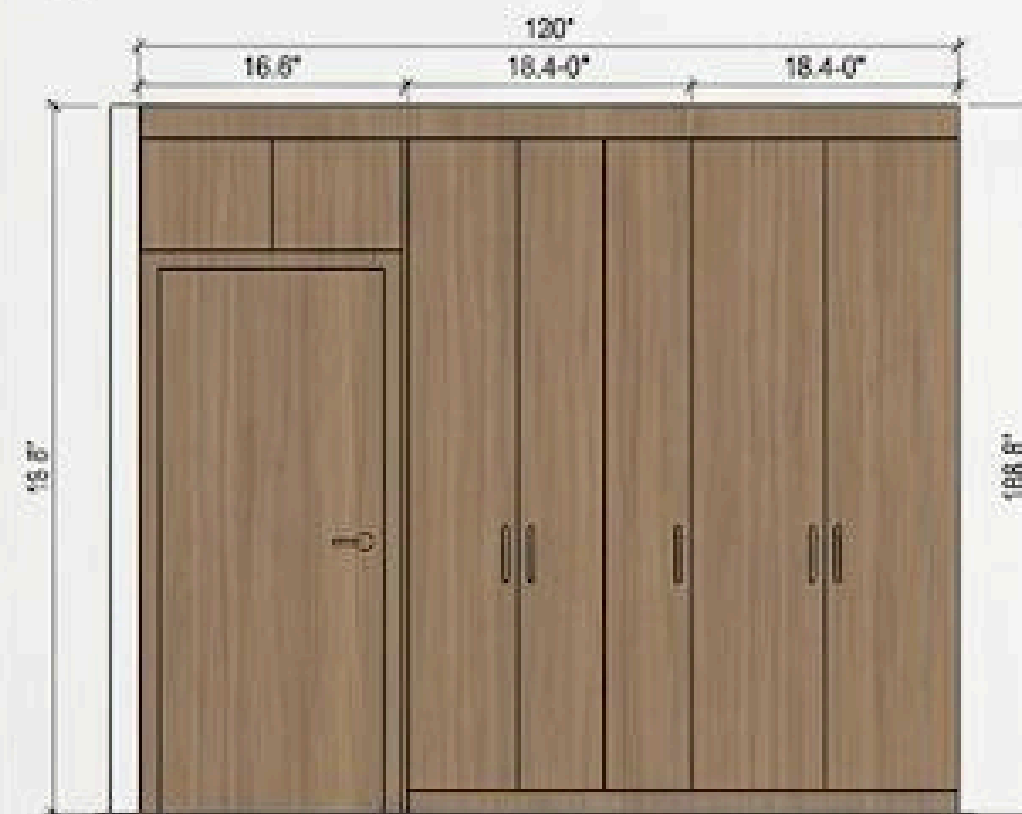
B/2 ELEVATION B: CABINET & DOOR WALL ELEVATION
